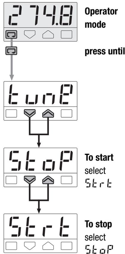
The green led **AT** goes on when the Fuzzy Tuning is in progress. At the end of this operation, the calculated PID terms parameter are stored and used by the control algorithm and the controller goes back to the operator mode. The green led **AT** becomes off.
