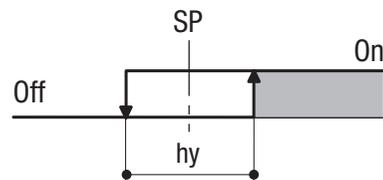
Control output hysteresis span, set in % of the full scale.
