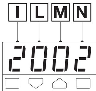
The configuration code can be displayed on the front panel, following the instructions at pag 19 section 4.2.2.
